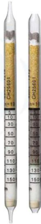
Figure 3: Drager glass tubes to test the concentrations of carbon monoxide [11].
